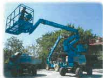
62呎, 橫伸40呎曲臂式升降台 62ft. Reach 40ft. Articulating Boom Lift (Diesel)
