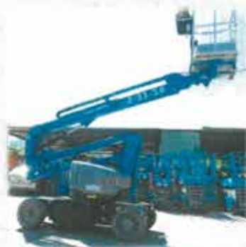
33呎電動曲臂 (淨重3噸) 33ft. Elect. Articulating Boom Lift (Net weight 3 ton)
